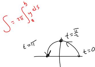
$$\begin{aligned} S &= \int_0^\pi 2\pi r \sin t \sqrt{r^2 \sin^2 t + r^2 \cos^2 t} dt \\ &= 2\pi r \int_0^\pi \sin t \sqrt{r^2} dt \\ &= 2\pi r \int_0^\pi r \sin t dt \\ &= 2\pi r^2 \int_0^\pi \sin t dt = -2\pi r^2 [\cos t]_0^\pi \\ &= -2\pi r^2 [-1 - 1] = 4\pi r^2! \end{aligned}$$
