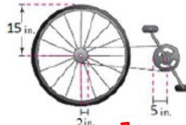
$$\left(\frac{1.4 \text{ rev}}{\text{sec}}\right) \left(\frac{5 \text{ rev wheel}}{2 \text{ rev pedal}}\right) \left(\frac{2\pi}{1 \text{ rev}}\right) (15 \text{ in}) \left(\frac{1 \text{ ft}}{12 \text{ in}}\right) = \left(\frac{7}{10}\right) \left(\frac{5\pi}{2}\right) \left(\frac{5}{12}\right)$$
